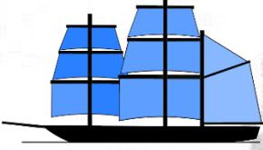
***Ship-built but converted to barque 543 tons Old Measure, 125' long x 30' 6" wide at her broadest point and 6' feet 8" 'tween decks.***
